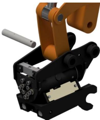
Position the link arm so that its pin bolt hole is flush with the mounting holes in the machine bracket (**Figure 2**).
