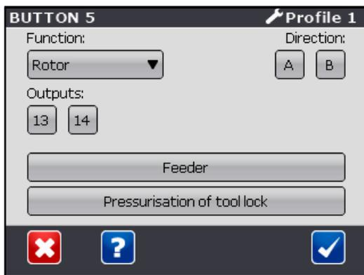
Here one can select which outputs must be activated together when the button is pressed. For each function in the dropdown menu, one must select whether the button should activate the function's A or B output.
