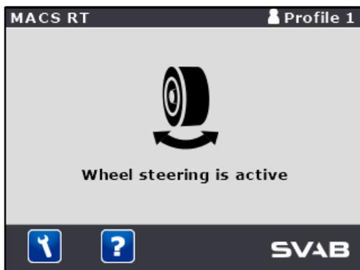
On the operating side, there will be an indication displayed when the wheel steering function is active.
