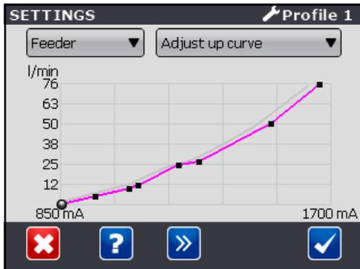
On the pages "Adjust up curve" and "Adjust down curve" one can edit the relevant curve.
