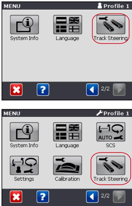
If the system is equipped with a track steering module, an icon for settings for this will be displayed under the main menu.
