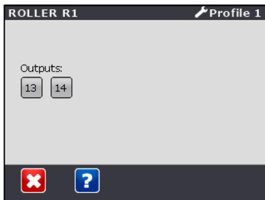
Here one selects which outputs must be activated together with the selected main function. "13" and "14" each represent an output in the GP1 unit.
