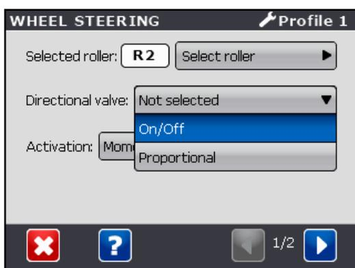
The system can be configured to use one of two different basic types of hydraulic valves, which is set by stating what type of valve controls the wheels' steering direction:
