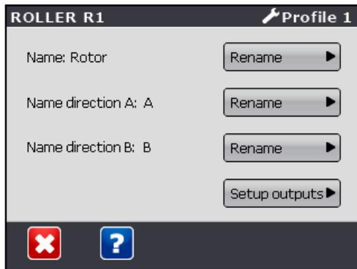
When one pushes a function's wrench button, one comes to a page where one can choose to rename the function and its directions, or continue to a page where one selects which extra outputs will be activated in conjunction with the function being run.
