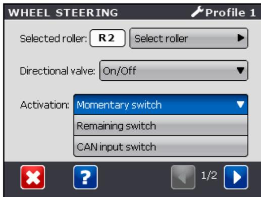
The system can be configured for different types of input signals for wheel steering activation:
