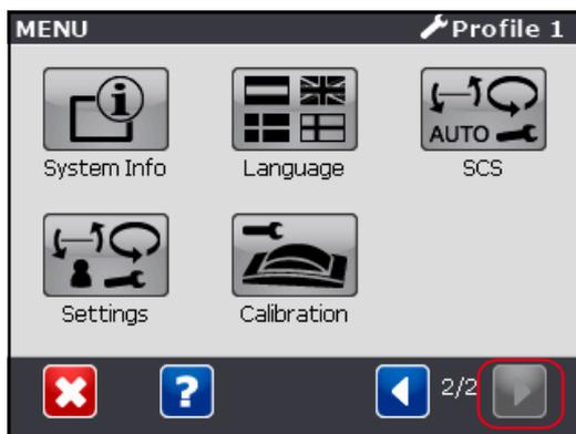
Unlock the service menu according to chapter 9.1. Select the last page in the main menu and then press the grayed out right arrow in the lower right corner, hold for five seconds.
